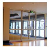
Steel profiles for non-rebated double acting swing doors in combination with fixed screen assemblies, providing up to 90 minutes fire integrity. Cold rolled steel profiles are partly welded and partly spigoted for assembly on site, with welds ground smooth prior to painting. Door leaves are fully welded for strength and rigidity.
