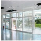
Steel profiles for fixed screen, door and window combinations providing up to 120 minutes fire integrity and smoke control. Cold rolled steel profiles are partly welded and partly spigoted for assembly on site, with welds ground smooth prior to painting.
