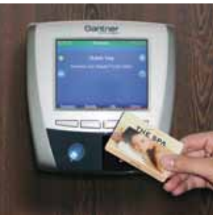
GAT-Lock 5010 with central information terminal: The compartment is opened by data carrier directly on the locker, whereas the central display provides information about which compartments are in use and which compartments are free.
