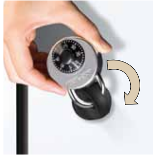
Safety turning bolt: The locking mechanism cannot be damaged by over-rotation since the lock cylinder does not snap into place until the padlock has been removed.
