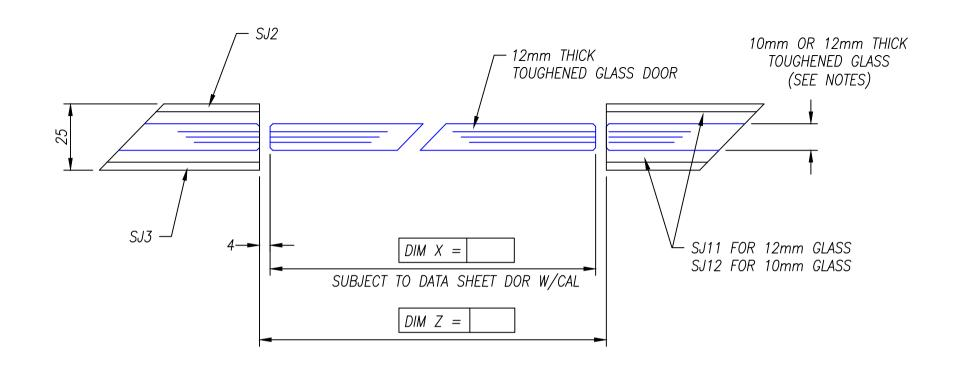
DIM X = DOOR WIDTHDIM Y = DIM X + 8
