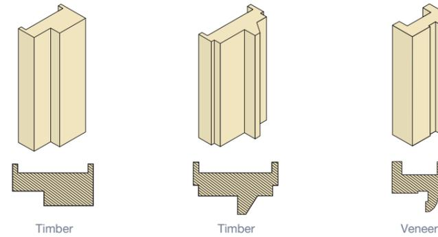
Code: A79 - Single acting door frame for 75mm system (FD30)
