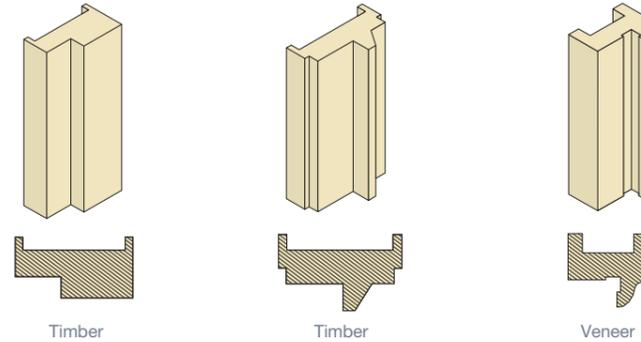
Code: A79 - Single acting door frame for 75mm system (FD30)
